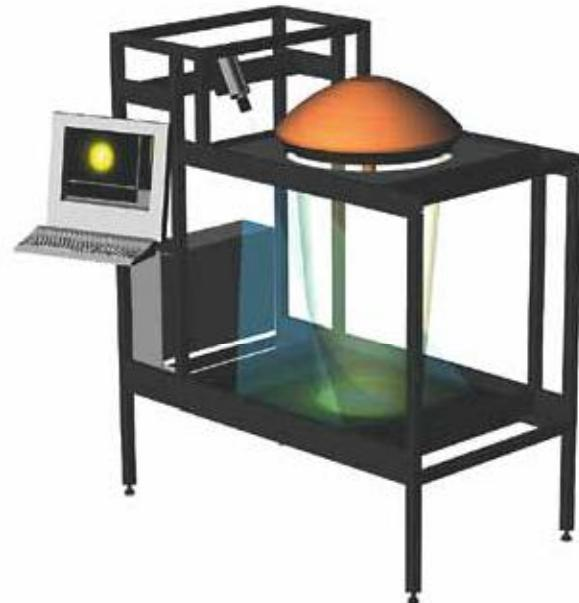
The measured illuminance distribution can be directly converted into the luminous intensity distribution and checked against the related standards. The measurement of the spatially taken chromaticity coordinate distribution is additionally enabled by the system enhancement. The measurement can be made from arbitrary inclined angles. The measurement algorithm provides for the geometric rectification of the measurement and directly delivers the evaluation of the luminance
