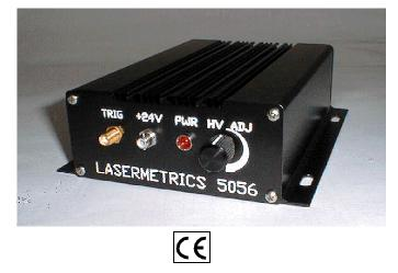
Referring to circuit diagram on page 2; when a trigger signal is applied, Side 1 switches from the pre-adjusted HV level to ground and then, between laser pulses, is allowed to recover to its original value.
