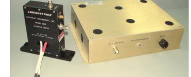
5250q-20 Laser Q-switch Drivers are valuable for laser Q-switching and cavity dumping. The drivers are effective in both intracavity and extracavity applications where a fast rise time pulse is needed. Typical rise times are <5 ns. The drivers provide the latest technology in reliable, solid state, high voltage switching design
