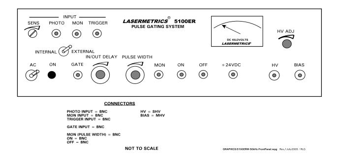
Figure 1. 5100ERW SYSTEM POWER SUPPLY / TIMING GENERATOR FRONT PANEL
