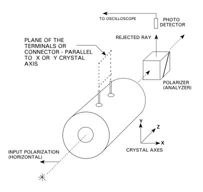
Figure 9. Arrangement of elements for detecting laser pulses with no voltages applied. Shows orientation of Pockels cell terminals with incoming plane of polarization. If the input plane of polarization is vertical and the cell is not rotated, the output polarizer (analyzer) can be rotated 90° around the propagation axis and operation will be identical. Typically, the X and Y crystallographic axes are optically equal and interchangeable.
