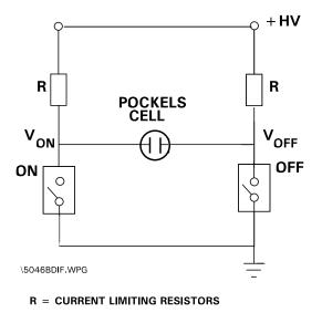
Figure 4 Differential Configuration
