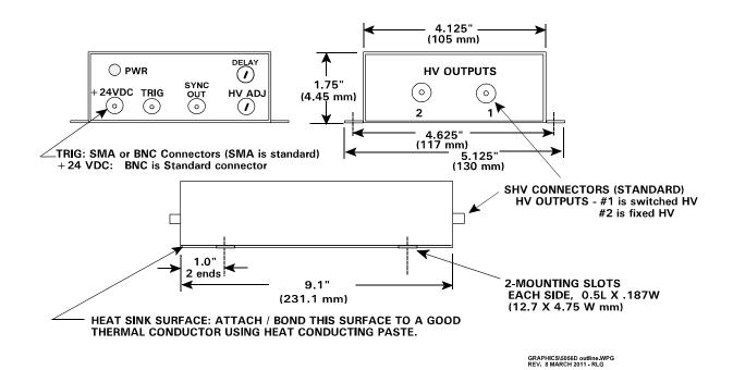
NOTES: The 5056D may be operated as a single ended driver. In this mode of operation, a DC high voltage is applied to the Pockels cell (PC) to attain a static ¼ or ½ wave retardation. The voltage may then be switched to the ground state. It will typically recover to the high voltage set point within 150 microsecond time period. This operation is set up as follows:
