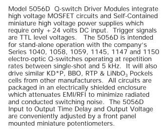
The 5056D features a balanced output, i.e., there are 2 independent output connections, one for each terminal on the Q-switch. The static, unswitched HV outputs have identical HV DC levels which produce a zero net differential voltage across the crystal.
